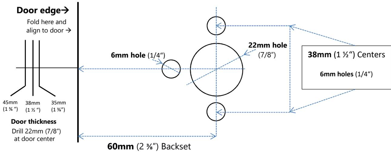
**Tubelatch** (to chisel out. Below diagram not to scale)
